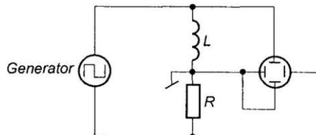
Fig. 1 Schematic configuration diagram for observations of current, voltage and phase trajectory in the *RL* circuit
