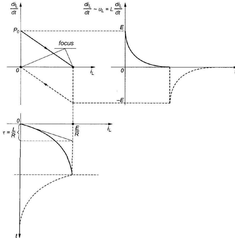
Fig. 4 The phase trajectory of the  $i_L$  current together with the time functions of  $i_L$  and  $u_L$
