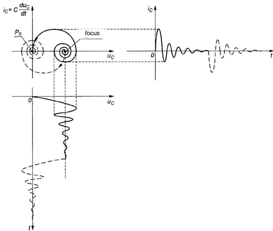
**Fig. 7** The phase trajectory of the  $u_C$  voltage together with the time functions of  $u_C$  and  $i_C$  in the oscillatory conditions in  $RLC$  circuit branch.
