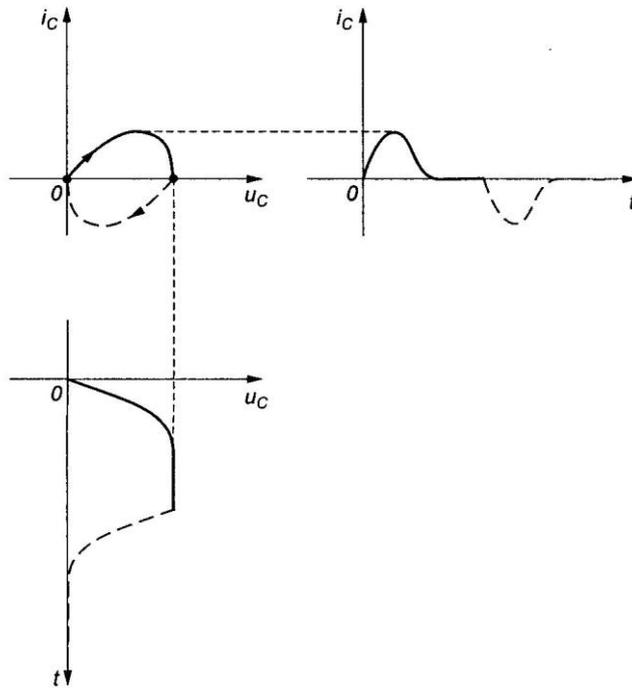
**Fig. 10** The phase trajectory of the  $u_C$  voltage together with the time functions of  $u_C$  and  $i_C$  in the aperiodic conditions in  $RLC$  circuit branch.
