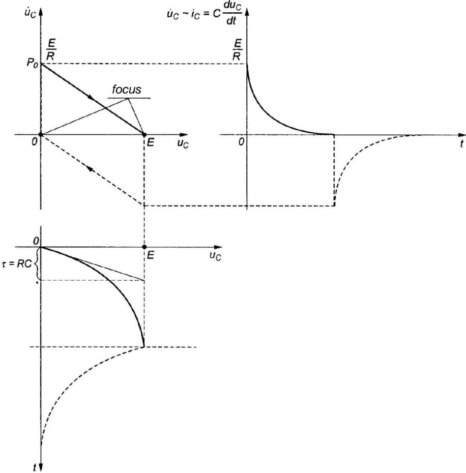
**Fig. 2** The phase trajectory of the  $u_C$  voltage obtained as the time functions of  $u_C$  and  $i_C$  match
