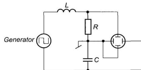
Fig. 5 Schematic configuration diagram of the  $RLC$  circuit for observations of the:
