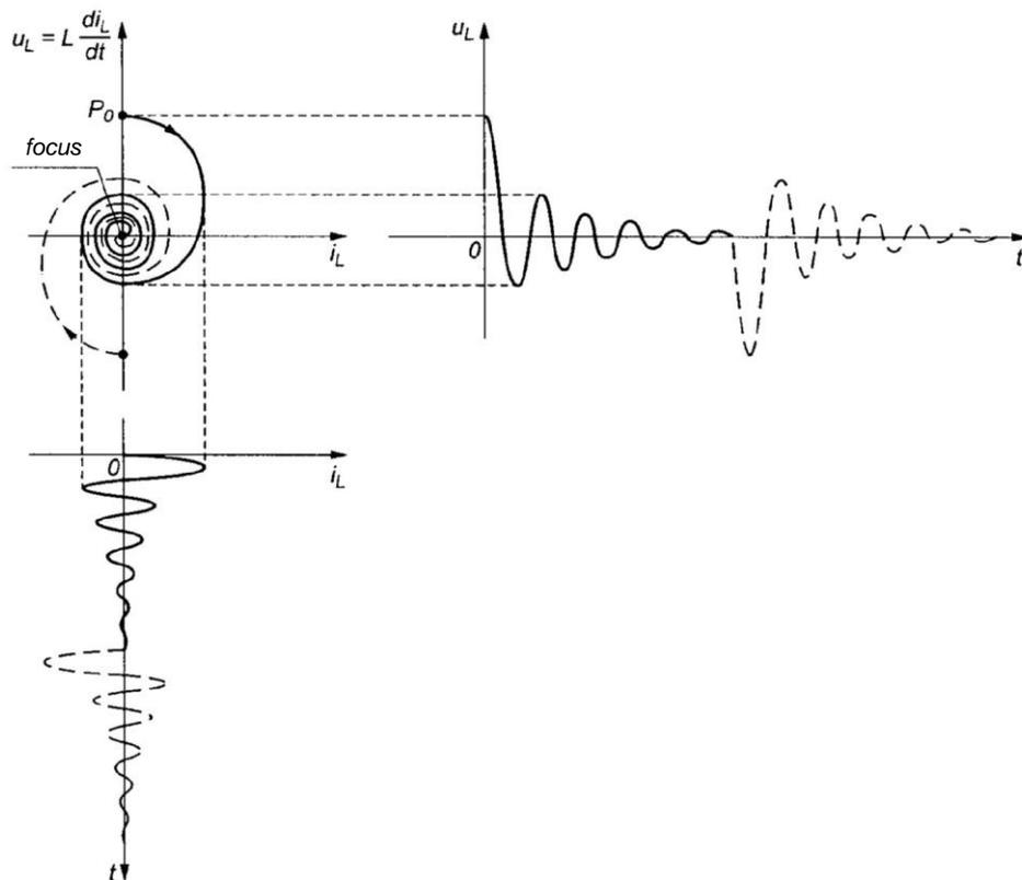
**Fig. 8** The phase trajectory of the  $i_L$  current together with the time functions of  $i_L$  and  $u_L$  in the oscillatory conditions in  $RLC$  circuit branch.
