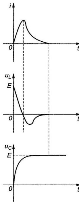
**Fig. 9** The time functions of the capacitance and inductance voltage and current in the *RLC* circuit branch during the transient state in the aperiodic conditions.
