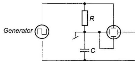
**Fig. 3 Schematic configuration diagram for observations of current, voltage and phase trajectory in the  $RC$  circuit**
