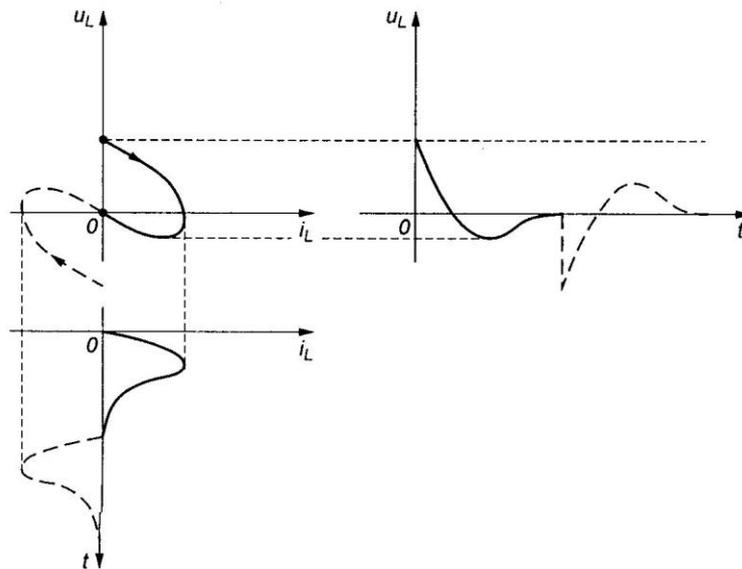
**Fig. 11** The phase trajectory of the  $i_L$  current together with the time functions of  $i_L$  and  $u_L$  in the aperiodic conditions in  $RLC$  circuit branch.
