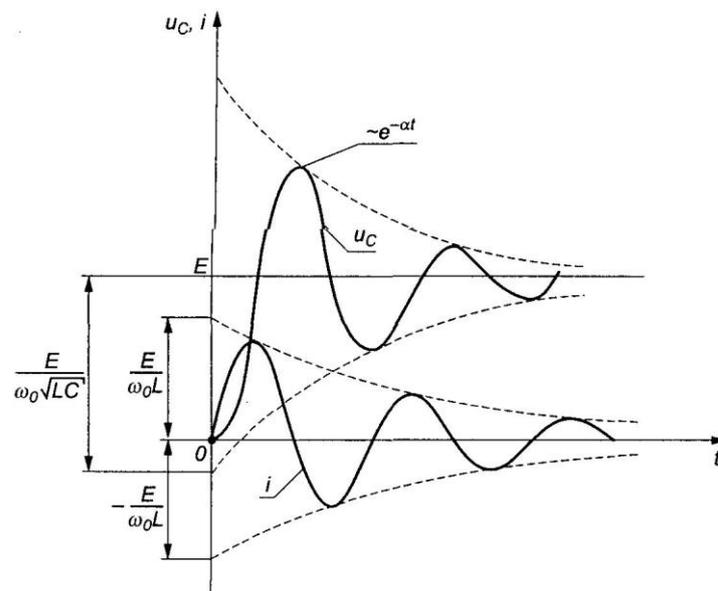
**Fig. 6** The time functions of the capacitance voltage and current in the *RLC* circuit branch during the transient state in the oscillatory conditions. The oscillatory attenuation of the functions is marked with the dashed lines.
