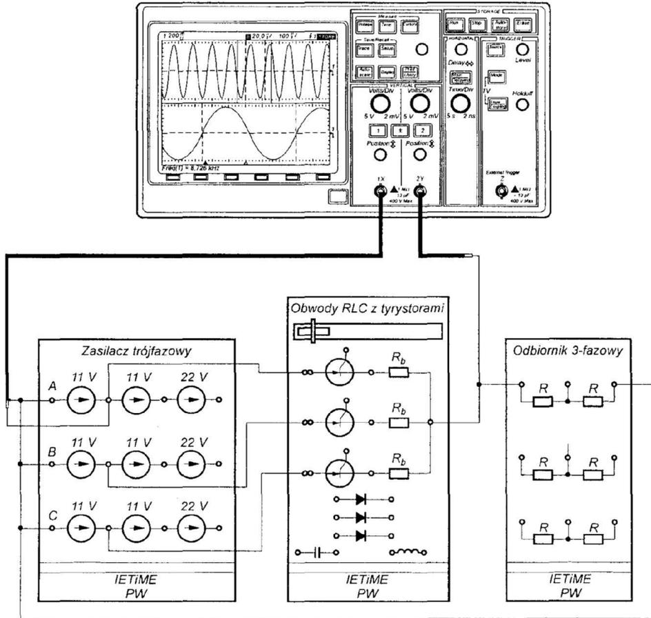
Fig. 3 Metering circuit configuration for examination of a three-phase, half-wave controlled rectifier with resistance load
