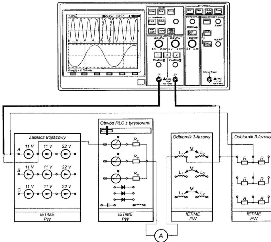
Fig. 1 Metering circuit configuration for examination of a single-phase, half-wave controlled rectifier with  $RL$  load
