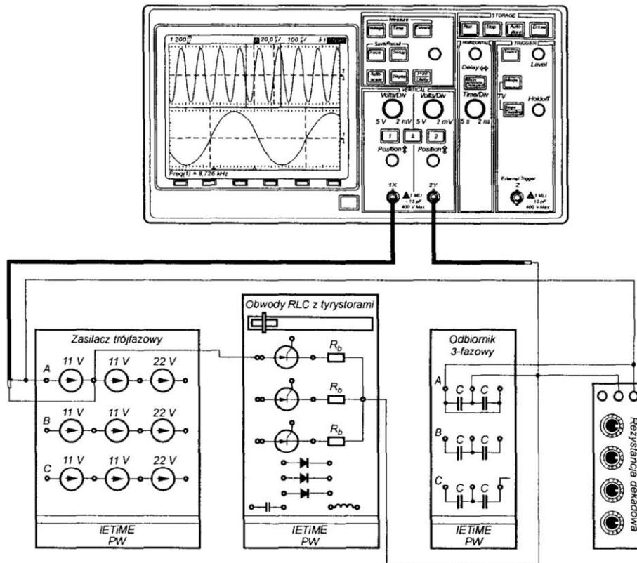
Fig. 2 Metering circuit configuration for examination of a single-phase, half-wave controlled rectifier with  $RC$  load
