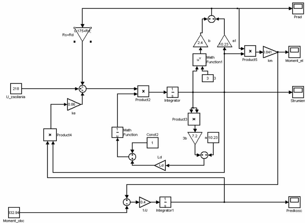
Rys. 1 The Simulink model of the series DC motor
